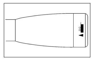
Press the button at the end of the shift lever to enable/disable the tow/haul mode.
